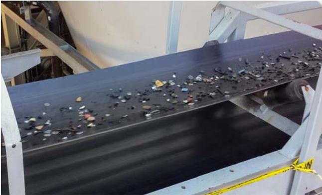
Figure 6: Glass, grit and other heavy contaminants removed from the test materials by the Wet Density Separation System (WDS).
