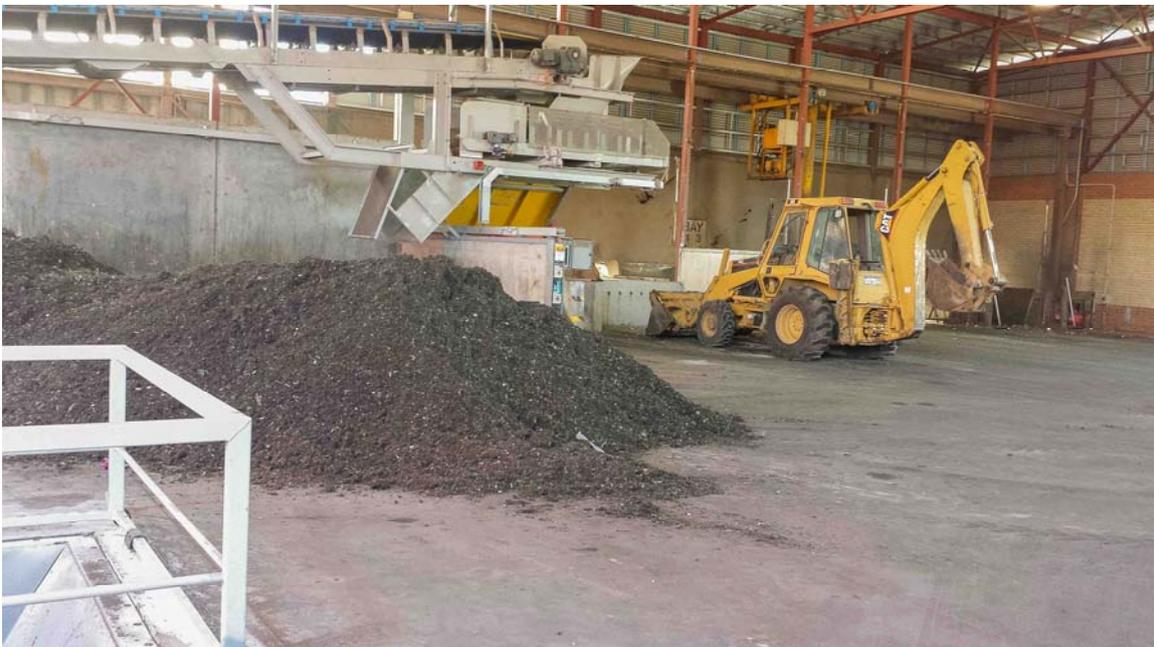
**Figure 4:** Test material on the transfer station tipping floor prior to introduction into the Material Recovery Facility (MRF).
